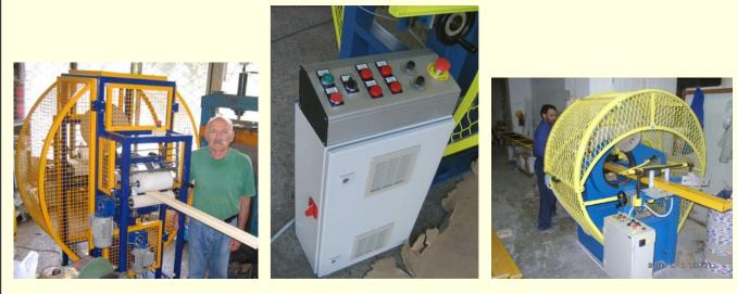
It takes 2 crepe paper or plastic band rolls simultaneously. Paper or Plastic Roll diameter: **500 mm** max, limited though by a maximum roll weight of 6 kg. Roll's width: 80 to 120mm. Roll's internal diam: 2 inches (50,8mm). Profile's bundle cross section: 340mm of diagonal. Advancement's speed: 5 to 25 m/min. • The machine includes one circular ring (350mm int.diam) revolving and driven by trapezoidal belts,
