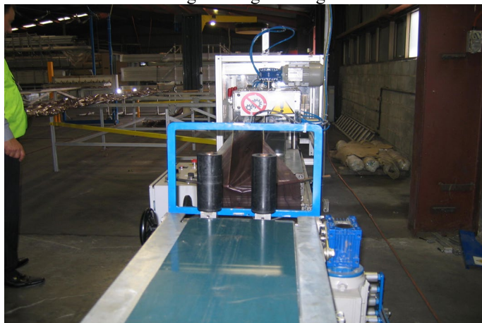
Loading belt and automatic lateral transfer at unloading towards Oven's truck loading
