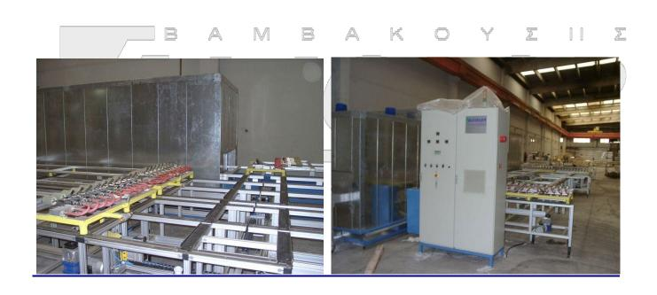
SUBLIDECOR 700 SUBLIBAG 3X10: Gas heated Plant with 3 detachable vacuum application Frames with 10 Aluminium 7 meters long Profiles each in a fully automatic movement. One Trolley is handling the 3 separate loaded Frames in and out the Oven. Production of up to 120 Profiles per hour.
