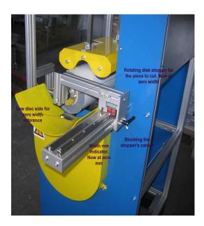
The machine cuts Rolls and Tubes of maximum outside diameter 400 mm and min inside diameter 75 mm:
