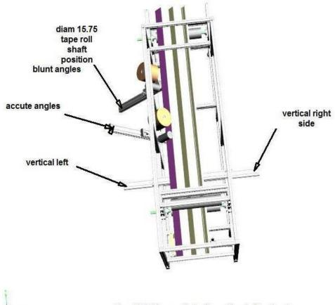
diam 15.75 tape roll shaft position is fixed, not sliding diam 15.75 tape horizontal roll shaft positions are not shown here
