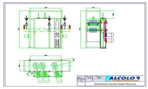
Above it is shown the general main machine arrangement. Shown also the possibility of disc packs orientation
