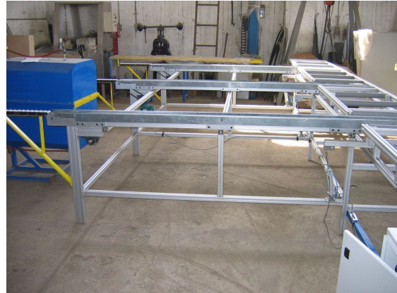
Total installed power 1,5 kw and production capacity up 3 ton/of aluminium profiles per hour
